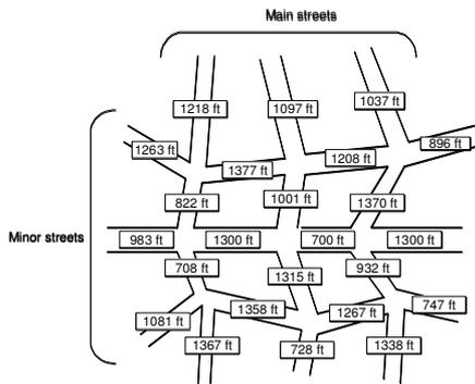
Figure 5: Link lengths of irregular grid network in experiment 2.
