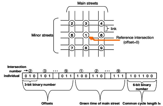
Figure 1: Grid network and coding method of control parameters.
