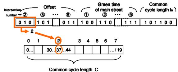
Figure 2: Calculating method of offsets and green time of main streets.
